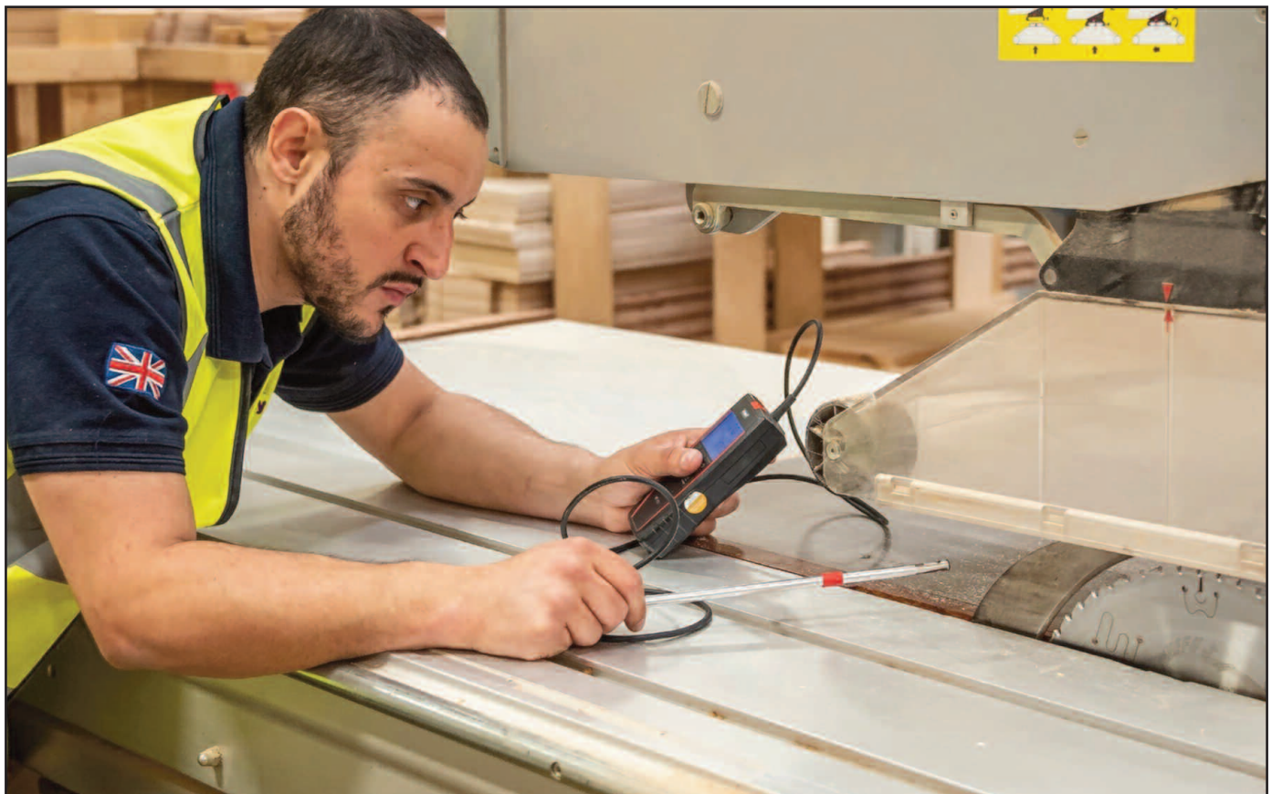
Testing LEV efficiency at source.
