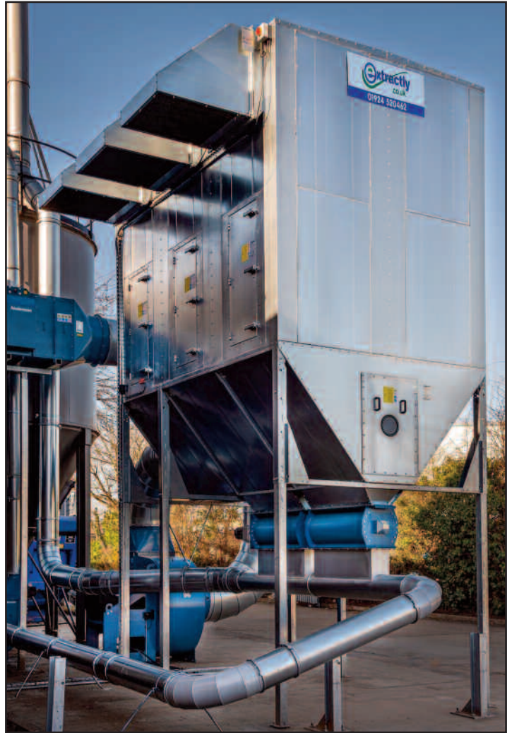
Nederman LBR-R SmartFilter with rotary valve discharge, 55 kW main fan and 15 kW transport fan.
