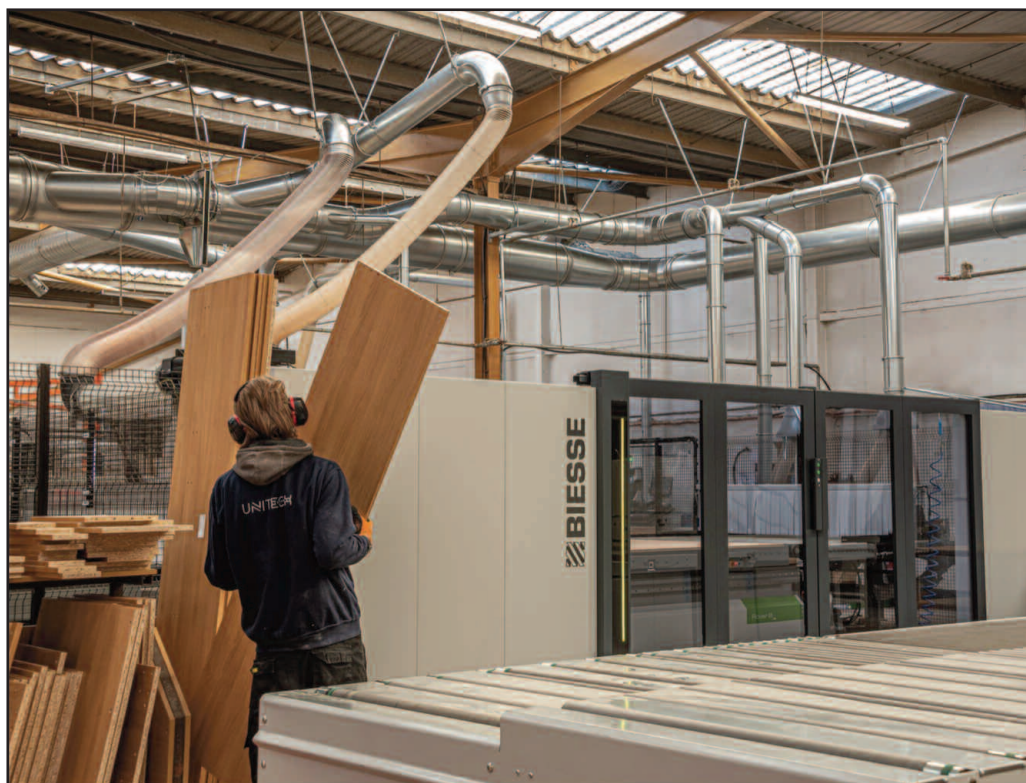
Installation of the new Biesse Rover B FT HD was the catalyst for upgrading the extraction system at Unitech Oxon Ltd.
