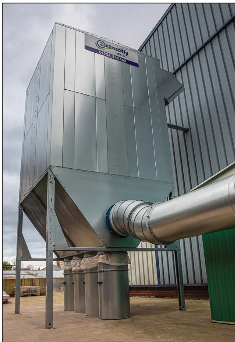
The 20,000 m 3 /hr capacity LBR-B SmartFilter with steel collection bins.
