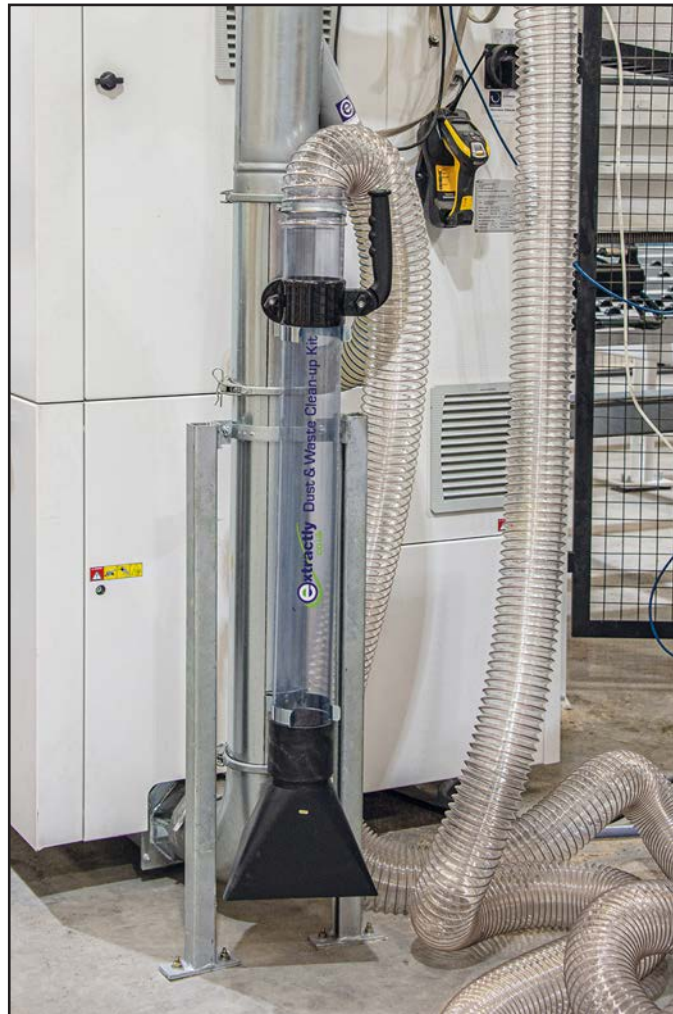
Extractly's 'Clean-up' tool accessory extracts directly to the main ductwork.
