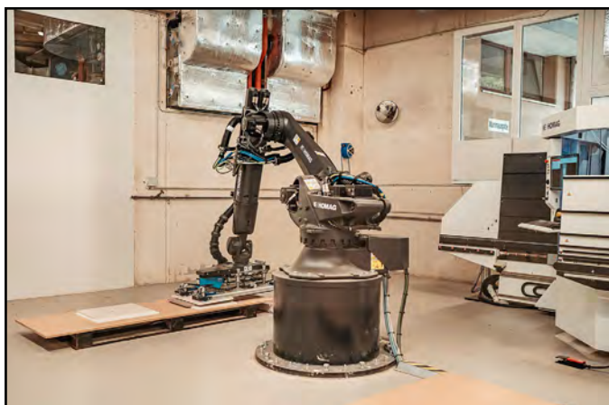
After gripping, the robot feeds the component into the CNC machining centres. Copyright: HOMAG.
