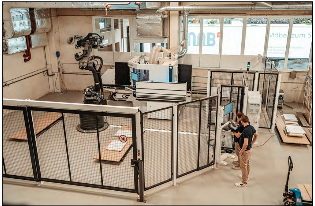
Robotic cell for fully autonomous machining of workpieces. Copyright: HOMAG.
