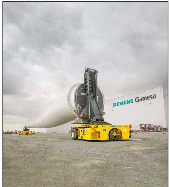
*Above: the newly-launched Combi-LC from CombiLift at Siemens Gamesa. The Combi-LC is designed to meet the load handling demands of largescale offshore wind manufacturers.*
